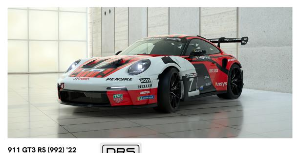
911 GT3 RS (992) '22 Displacement: 3,996 cm3 Drivetrain: RR Max. Power: 517 hp / 8,500 tr/min Max. Torque: 47,4 kgfm / 6,500 tr/min Weight: 1,450 kg Aspiration: Atmospheric engine
